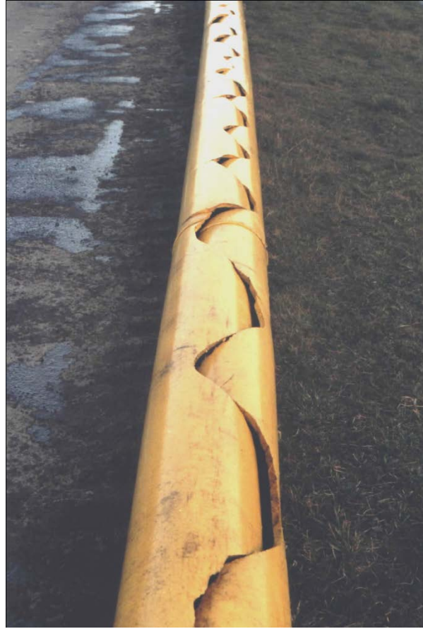
Figure G.1RCP in 315 mm SDR 17.6 PE80 pipe
